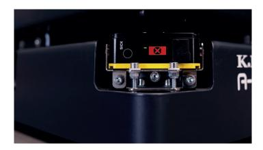
**MULTIPLE SCANNERS** to make the A-MATE® a 360° safe mobile robot
